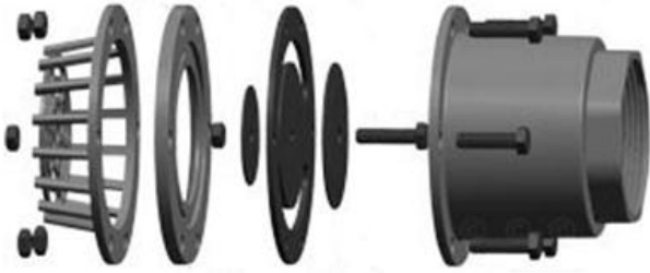
Fig 1: Exploded view of Commercial Flap Non-Return Valve
