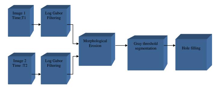
Fig.1 Flow chart of the proposed change detection algorithm.
