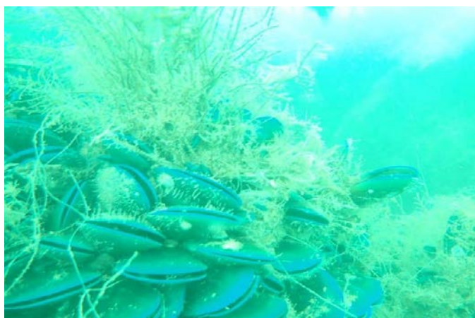
Figure 4: Bio growth inside strainer
