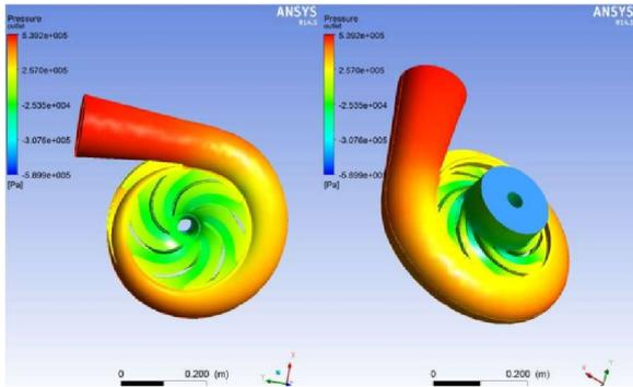
Fig4. Pressure counters flow through the pump
