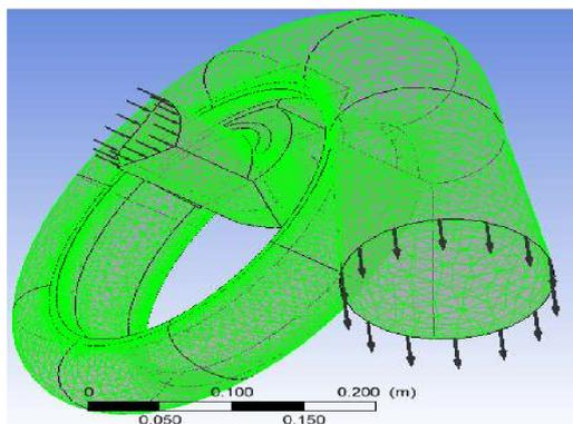
Fig1.: Mesh profile for centrifugal pump.
