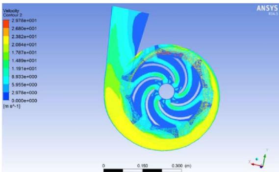
Fig5: Velocity counters flow through the pump in the 3D mid plane view at design value of the flow rate.
