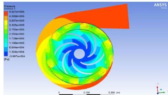
Fig2: Pressure counter flow through the pump in the mid plane view for Q = 36 m³/kg
