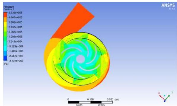
Fig3: Pressure counter flow through the pump in the mid plane view for Q=280m³/kg (At design value of the flow rate)
