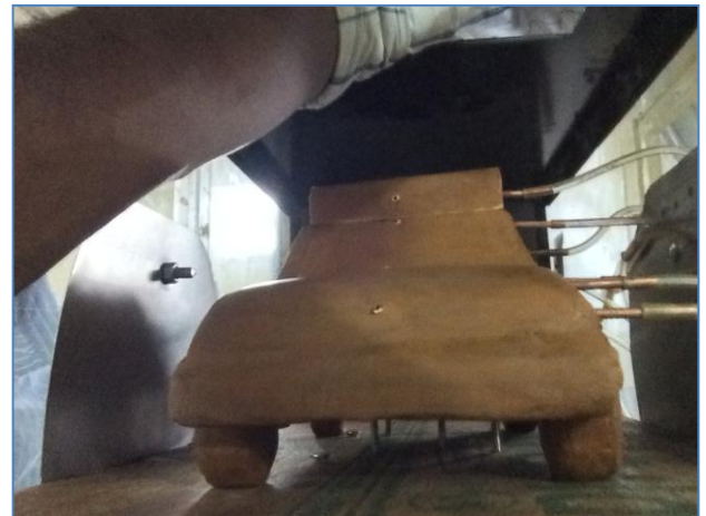
Figure 15: Experimental setup of car model with a drag breaking system
