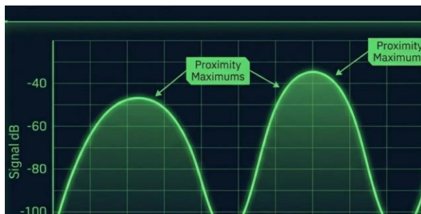
Fig. 3: Signal strength variation and illustrated handover execution points in the project scenario.
