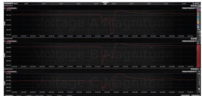
Fig.(7): 400 kV Farakka Bus voltage
