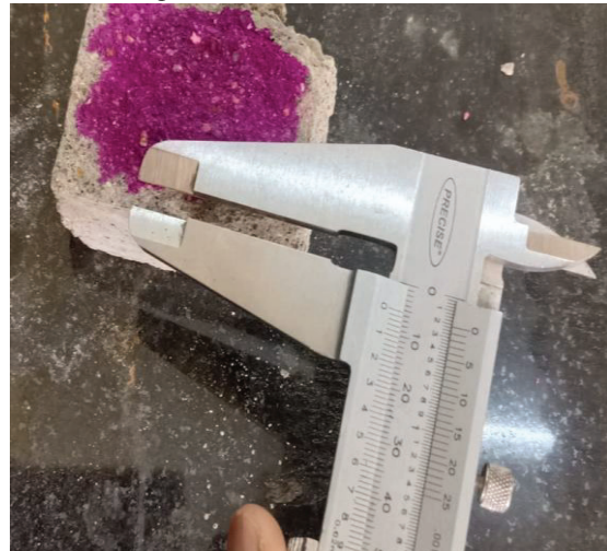
Fig.6(c) Carbonation depth measurement using Vernier Caliper
