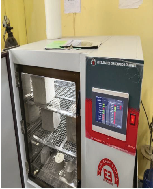
Fig. 3 Accelerated Carbonation Chamber Apparatus
