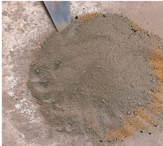
Fig. 5(a) Mixing of cement, sand and rice husk ash.
