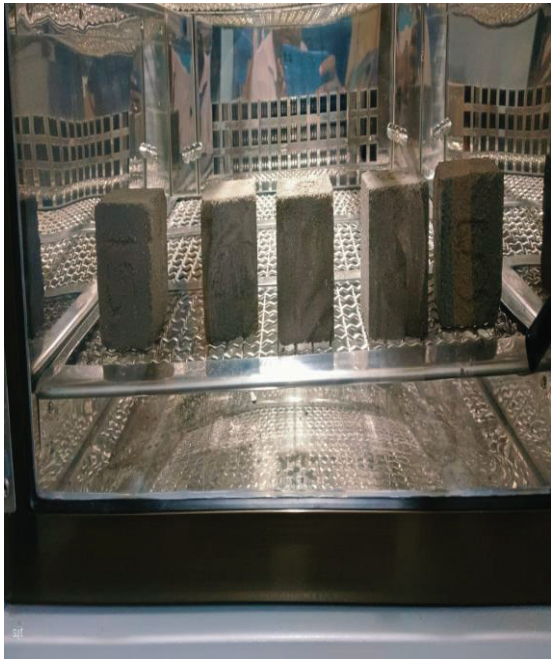
Fig. 1 Sample Placement in Accelerated Carbonation Chamber
