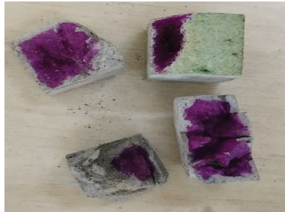
Fig. 6(a) Carbonation test using phenolphthalein indicator
