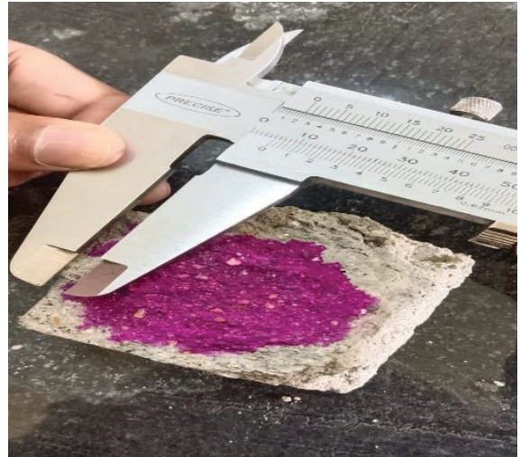
Fig.6(c) Carbonation depth measurement using Vernier Caliper
