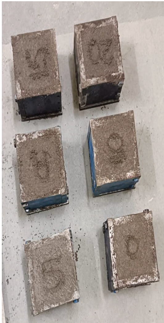
Fig. 5(b) Mortar Cube Sample Preparation with binary combination of cement and replacement of rice husk ash with variation of 5% from 0 to 20%.
