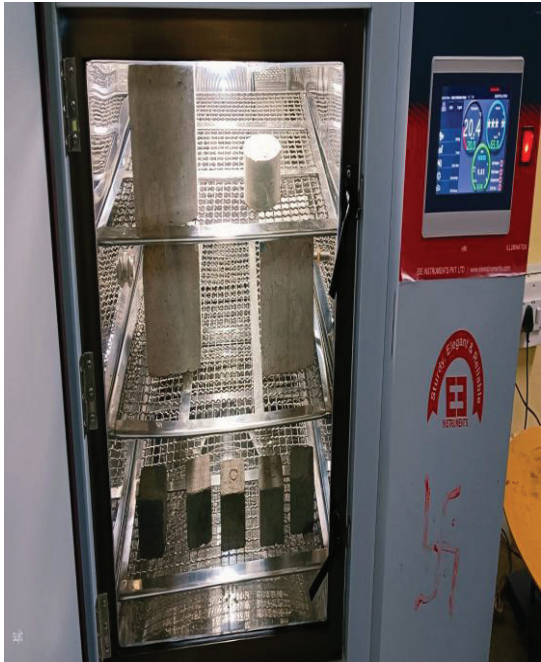
Fig. 2 Carbonation of Concrete Samples
