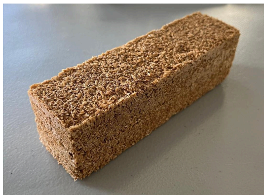
Fig. 5. Final rice husk-wax biobrick after 12-hour air setting, fully solidified and ready for mechanical testing.
