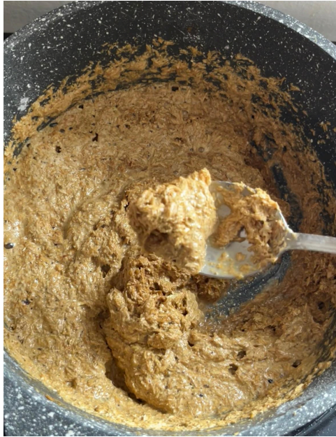
Fig. 3. Shredded rice husk is then incrementally added along with lime, and the mixture is homogenized to ensure consistency
