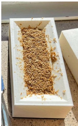
Fig. 4. Layer-by-layer pouring of the mixture into standardized molds with manual compaction.
