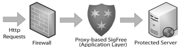
“Figure.1 MCAIDS is an application layer signature free blocker between the protected server and the corresponding firewall”
