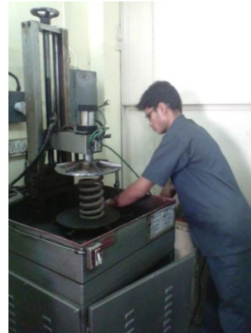
Figure 3. Checking for surface cracks by exposing to UV lights.
