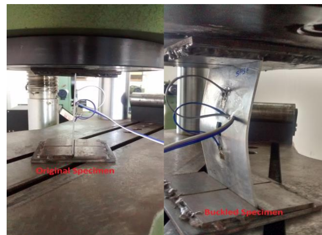
Figure 7: Typical buckled shape of isotropic plate specimen
