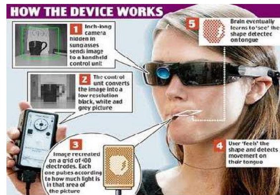
Fig.6 Working of Brain port device
