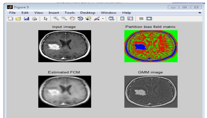
Fig 4.2.4. Illustration of Brain images partition bias field, estimated FCM, Gaussian Mixture Model image segmentation results.
