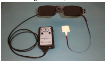
Fig.1: A Haptic Feedback device The base unit has features like zoom control, light settings control and intensity. Using these controls, users
