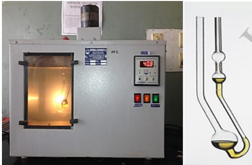
Figure-5: Kinematic viscosity bath Instrument with cannon fenske tube
