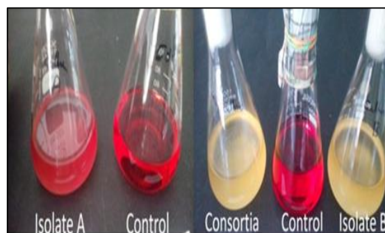
Fig. 3 Dye decolorization by isolated strain A, strain BPL and consortia of strain A and strain BPL with reference to control
