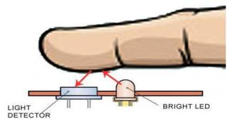
This circuit made from an infrared phototransistor and infrared LED. This transducer works with the principle of light reflection, in this case the light is infrared. The skin is used as a reflective surface for infrared light. The density of blood in the skin will affect on the IR reflectivity. The pumping action of heart causes the blood density rises and falls. So that we can calculate the heart rate based on the rise and fall of intensity of infrared that reflected by skin.
