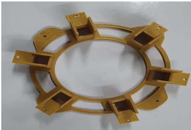
Figure 2 : 3D printed cuvette holder
