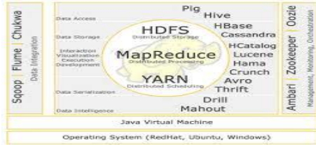
Fig 2. The image show the hadoop technology stack. hadoop core/common which consists of HDFS which is a programmable interface to access stored data in cluster.
