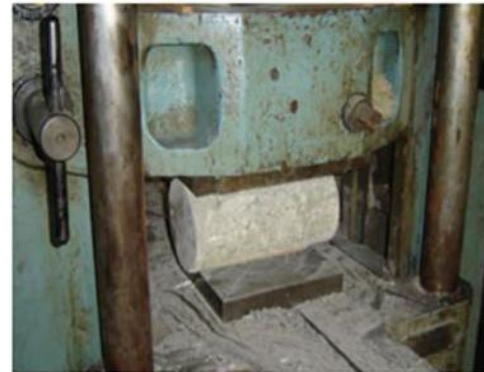
Figure 4. Split Tensile Testing.
