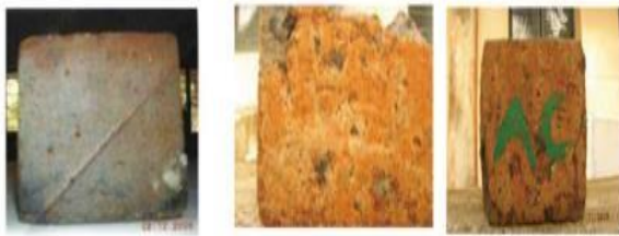
Figure.1. (a) Ordinary Concrete, (b) RHA Based concrete against acid attack [8]
