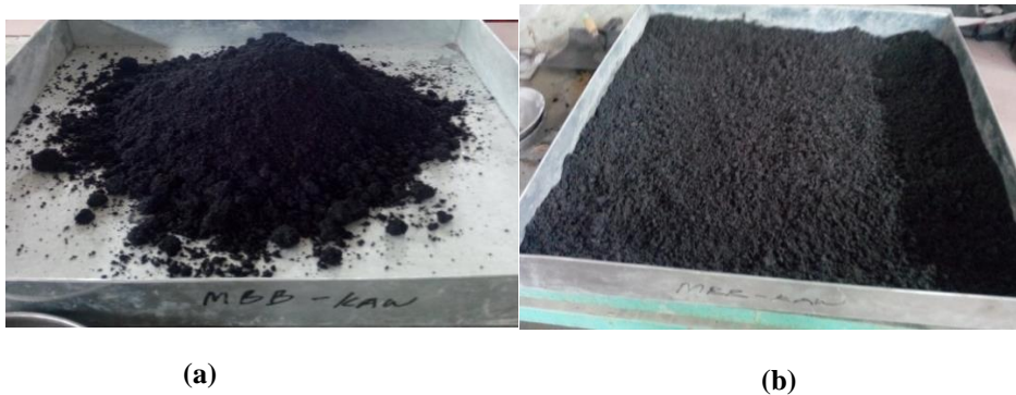
Figure 2: Soaked and Treated (TCR) crumb rubber aggregate.
