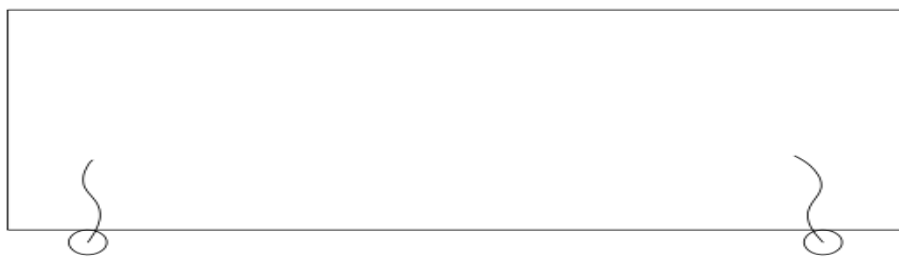
Figure 5: First mode of failure showing hairline cracks at the supports only
