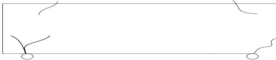
Figure 6: Final failure mode showing wider cracks and peeling at the supports
