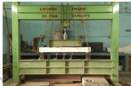
Fig. 3 Test set-up under loading frame
