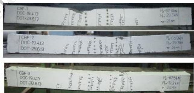
Fig.4 The cracking pattern of beam CBFs.
