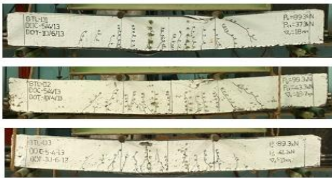
Fig. 7 The cracking pattern of beam BTLs.
