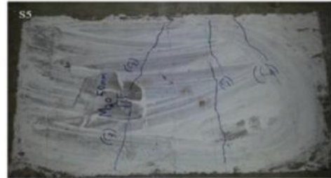
Crack pattern of slab M 20 50mm thickness 1% fiber
