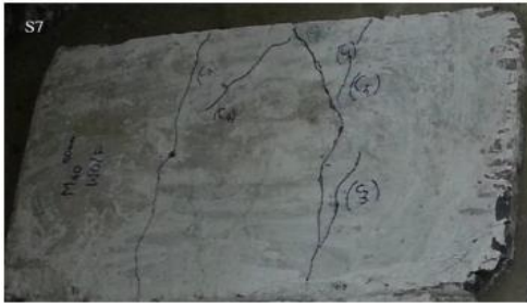
Crack pattern of slab M 40 50mm thickness without fiber
