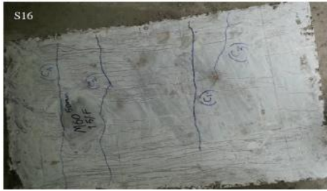
Crack pattern of slab M_{60} 50mm thickness 1.5% fiber
