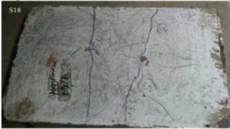
Crack pattern of slab M_{60} 75mm thickness 1.5% fiber
