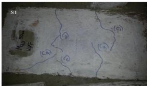
Crack pattern of slab M 20 50mm thickness without fiber
