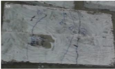
Crack pattern of slab M 40 75mm thickness without fiber
