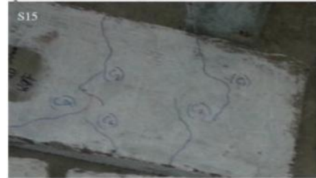
Crack pattern of slab M 60 75mm thickness without fiber
