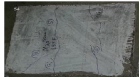
Crack pattern of slab M 20 50mm thickness 1.5% fiber
