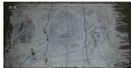
Crack pattern of slab M 60 75mm thickness 1% fiber
