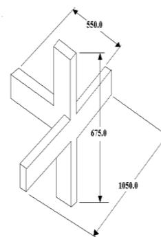
Fig.1 Specimen details
