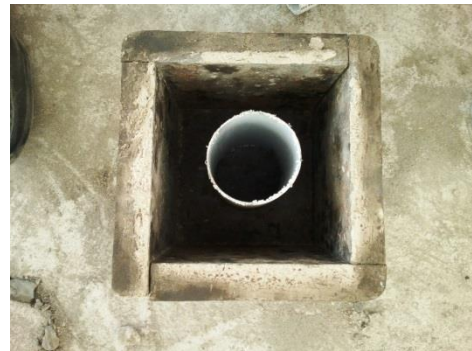
Fig2 (b) 4.5cm pipes in concrete cube
