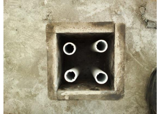
Fig2 (a) 2.5cm pipes in concrete cube
