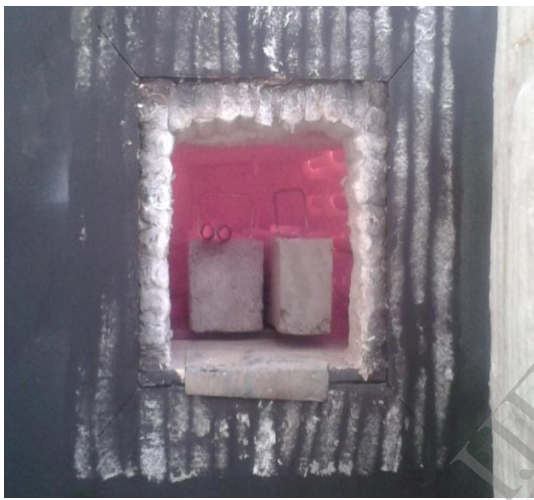
Fig. 1: Beam exposed for Heating
