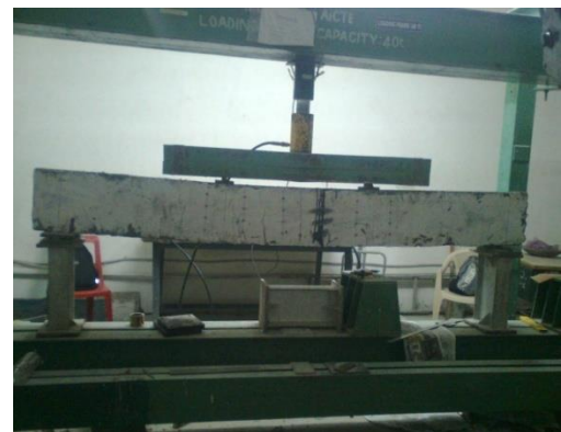
Fig. 3 Deflected profile of beam under symmetric loading
