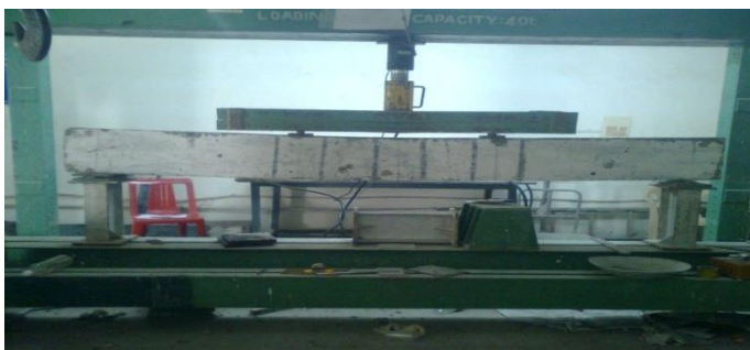
Fig. 1 Concrete beam casted using coconut shell as coarse aggregates
