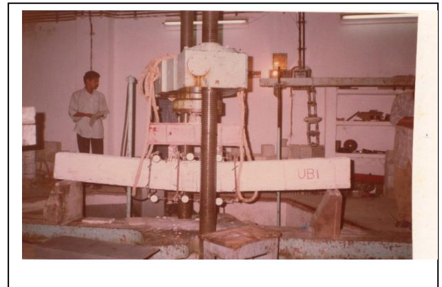
Fig.3. Photograph with the curvature meter
