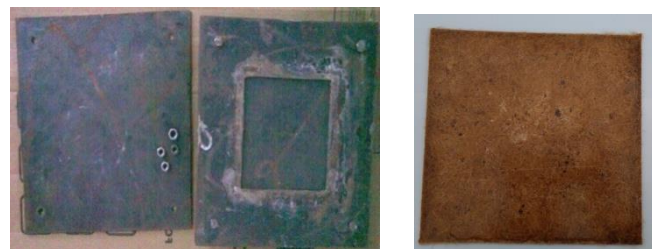
Fig 2.2 & Fig 2.3 Compression moulding Die & Fabricated composite plate
