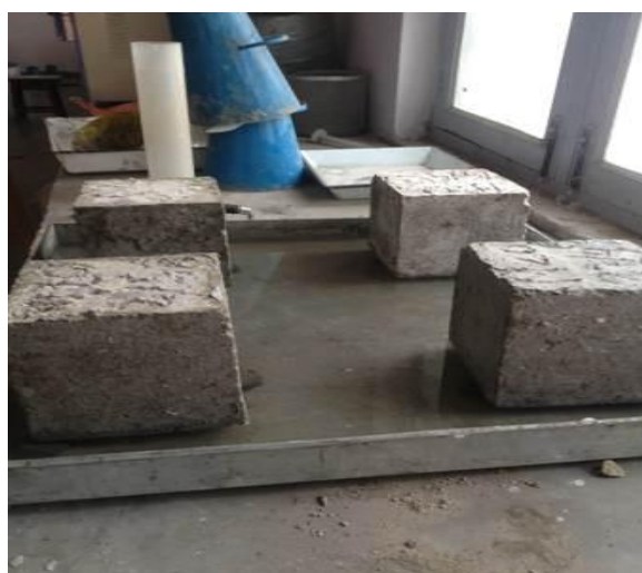
Fig. 1 Capillary Absorption Test
