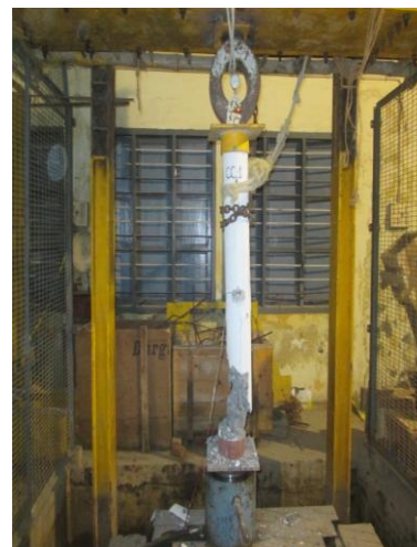
Fig.6. The Ultimate crack on the conventional column
