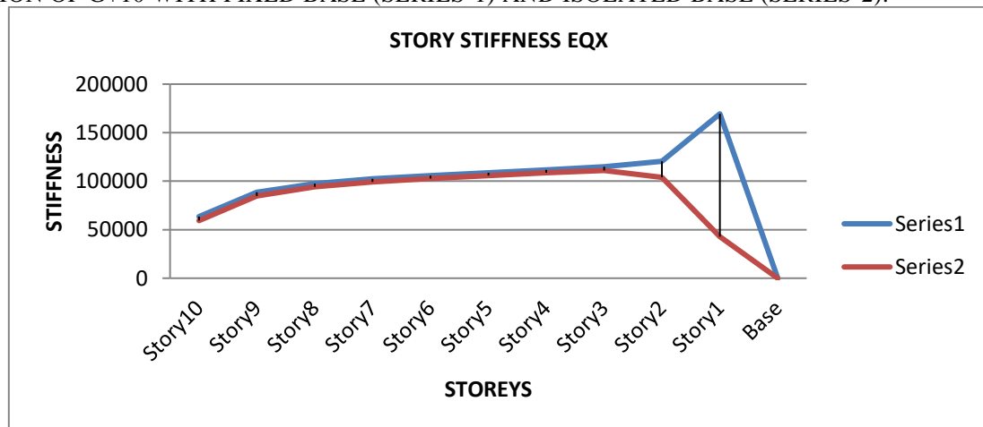
STOREY STIFFNESS COMPARISON OF G+10 WITH FIXED BASE (SERIES-1) AND ISOLATED BASE (SERIES-2).
