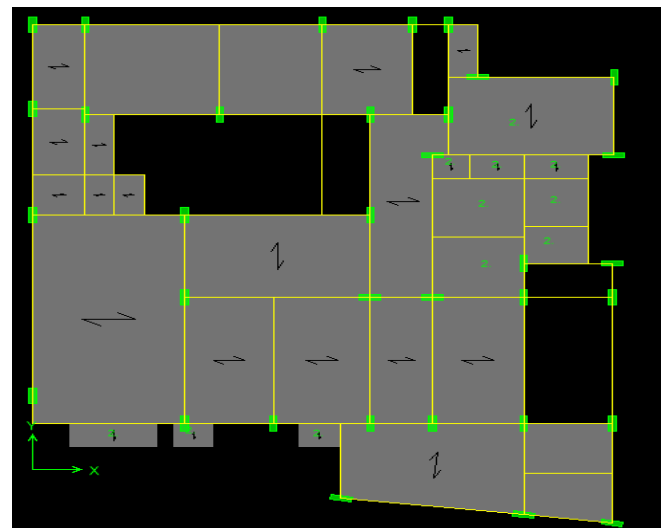
Fig No.7 First Floor Live Load
