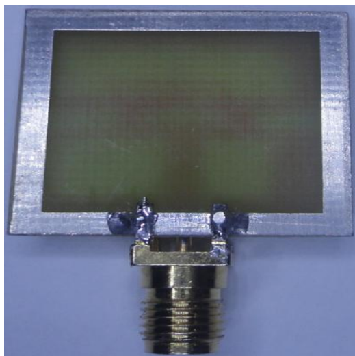
Figure 4. Fabricated U-L shaped antenna with wide slot in the ground plane
