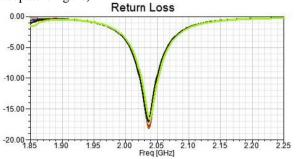
By care ful absorving the return loss curve, we can see merged return loss curves. There is an increment in the operating band width as the patch width is increasing and also simultaniously the return loss value is decreasing which indicates maximum amount of power is applied at input is transferred to out.
