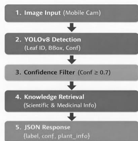
Fig. 1: Architecture of the proposed Ayurvedic Plant Identification System
