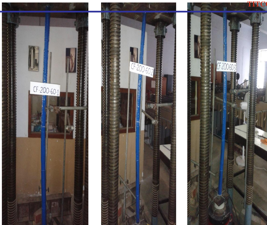
Fig. 6. Failure of CF-200-60 Specimen
