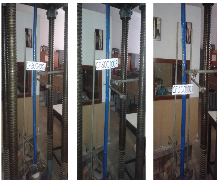
Fig. 7. Failure of CF-300-100 Specimens
