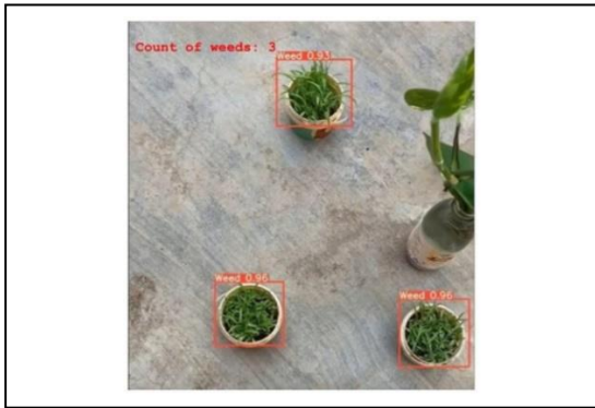
Fig.9 Weed count of 3 detected in image
