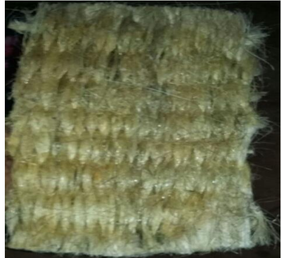
Figure 3. Sisal reinforced epoxy floor mat structure
