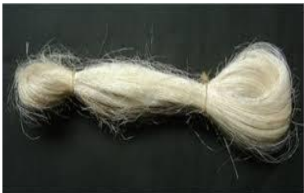
Figure 2. Raw Sisal Fiber
