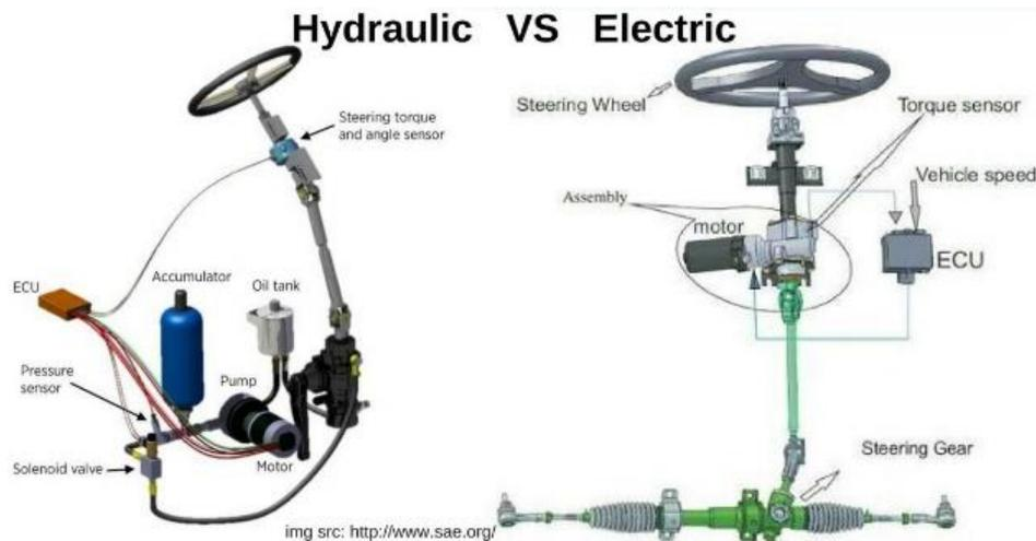
Development in the field of Steering system can be seen as the systems are now Electric Dependent rather than Hydraulic Dependent.
