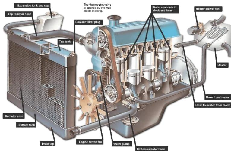
An Engines Cooling System using Radiator & other Equipment's like sensors used in modern Cars. In engines with small capacity the cooling process is done only by the air and thus to carry out this, the engines have fins around them which increases the area of contact of the engine with air. Hence the engine is cooled only by air. This system is used in lawnmowers and small capacity motorcycles etc.
