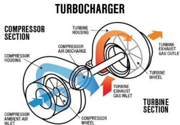
A Turbocharged System using Turbine and Suction Turbos.
