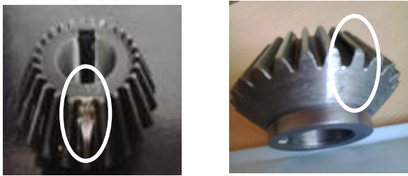
FIGURE VI. GEAR TOOTH BREAKAGE AND FACE WEAR
