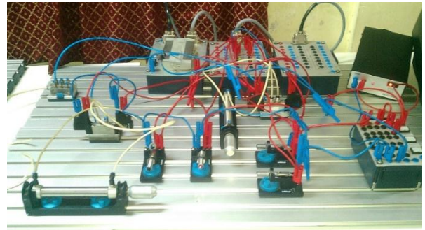
Fig 9: Inputs and Outputs of PLC for automation of Injection Moulding process
