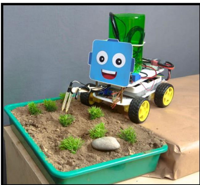
Fig. 3. Smart phone controlled Agricultural Robot for automatic irrigation system [6]
