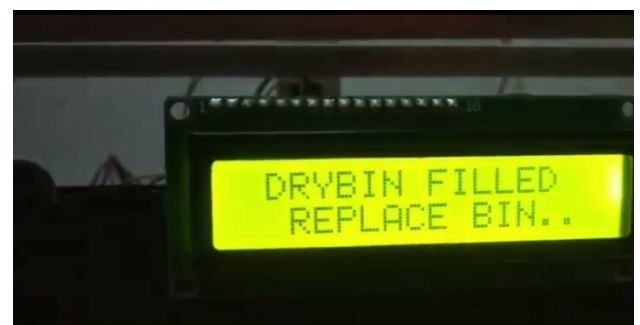
Fig.12. Message displayed to replace the bin as the dry bin is filled.
