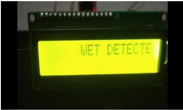
Fig.13. Message displayed that waste detected is wet in condition.
