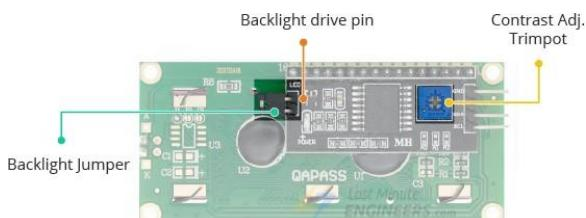
In addition, there is a jumper on the board that supplies power to the backlight. To control the intensity of the backlight, you can remove the jumper and apply an external voltage to the header pin that is marked as 'LED'.
