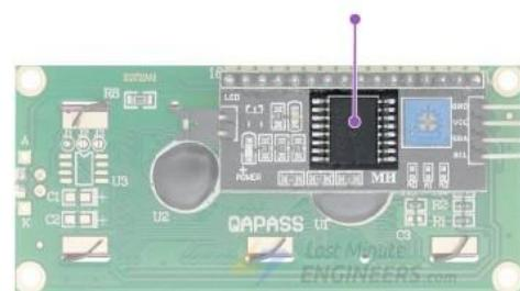
The board also comes with a small trim pot to make fine adjustments to the contrast of the display.
