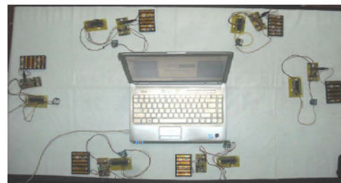
Fig.2 WSNs implemented in hardware with six sensor nodes.
