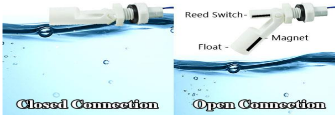
Fig2.5. float level switches
