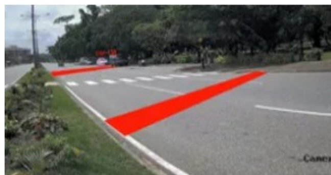
Fig. 3. Representation of the reference lines and the vehicle's path, illustrating how intersections are detected
