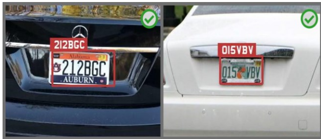
Fig. 4 Illustration of OpenALPR in action
