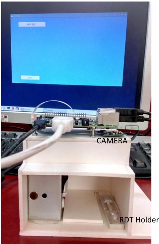
Fig. 2: Complete setup along with RDT holder and display
